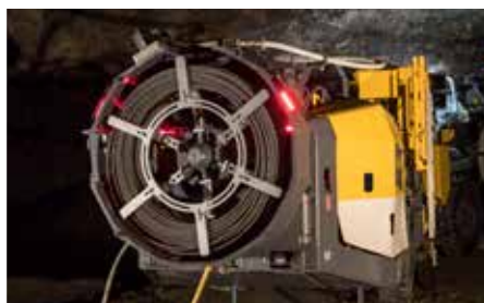
The machine has 500 kg of dry cement and approximately 775 m of 15.2 mm diameter bolting cable storage capacity.
