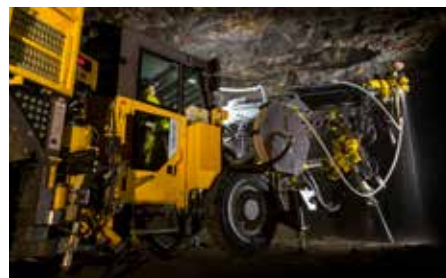
With a hole diameter range of 51-76 mm and 20 m mechanized drilling hole depth, Cabletec M can also be used as a secondary production drill rig.
