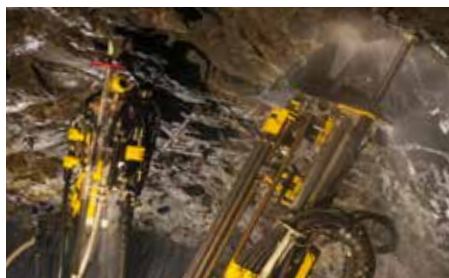
The fully mechanized drilling system of Cabletec M is taken from the well proven production drill rig Simba S7.
