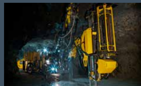
The fully mechanized drilling system of Cabletec E is taken from the well proven production drill rig Simba ME7.
