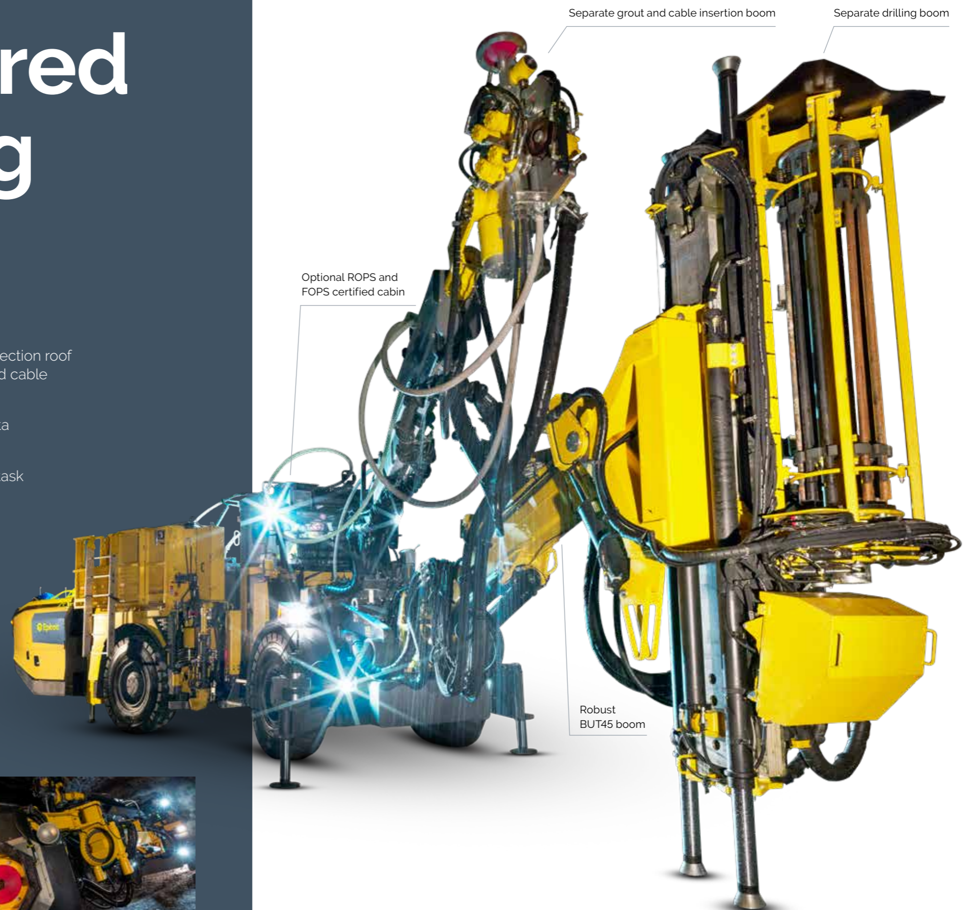
With a hole diameter range of 51-76 mm and 32 m mechanized drilling hole depth, Cabletec E can also be used as a secondary production drill rig.
