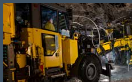
The machine has 1 000 kg of dry cement and approximately 1 700 m of 15.2 mm diameter bolting cable storage capacity.
