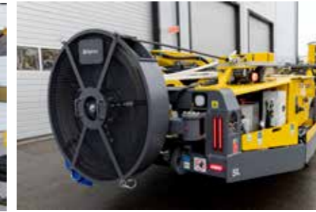
The machine has 150 kg of dry cement and approximately 150 m of 15.2 mm diameter bolting cable storage capacity.
