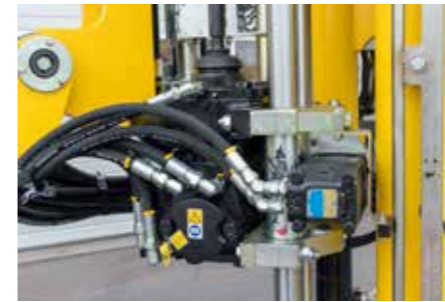
Ultra short COP 628 rock drill allows a reduced total feed length needed for low profile operations.
