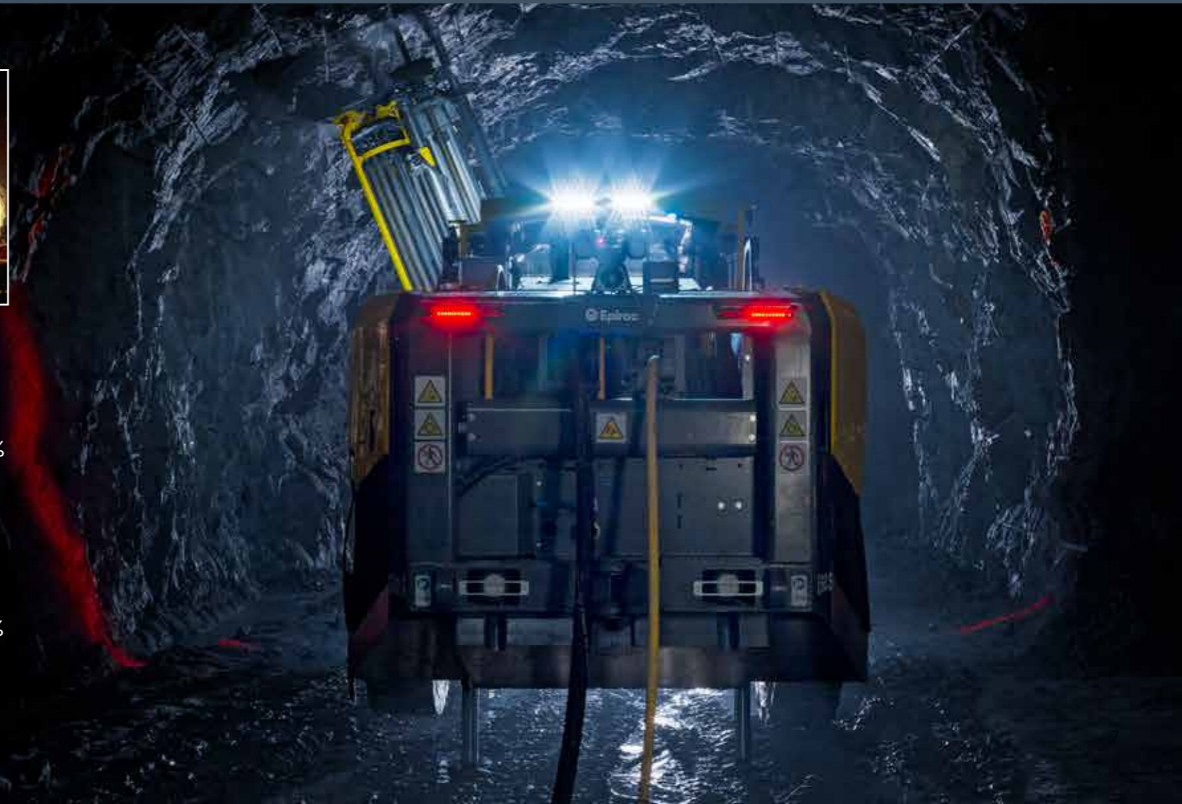
Total station navigation and Simba COPROD drill rig at Pucobre mine.
