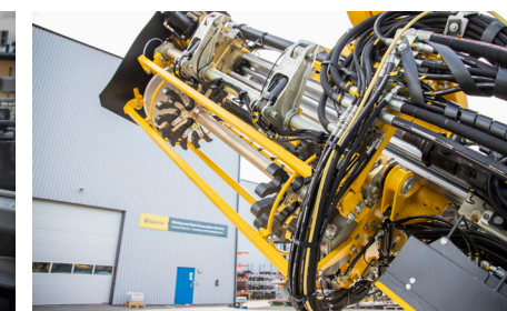
The carousel on the Simba E60 S rig has received a facelift compared to its predecessor. This improvement includes a new three-way cylinder replacing the hydraulic motor, improved material for the gripper arms and a new design for the drill steel grippers. The new drill steel support cylinders secure a solid grip when adding/removing drill steel during drilling.
