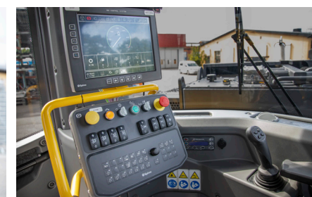
New touch screen and centralized buttons give the operator a better overview. The Carrier Control System (CCS) means increased effectiveness and is an enabler for future automation development.
