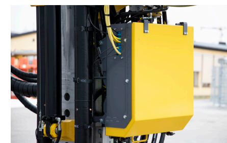
New smaller hydraulic box with improved sealing to prevent water entrance, overall resulting in better serviceability.
