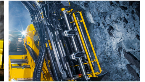
The carousel on the Simba M40 S rig has received a facelift compared to its predecessor. This improvement includes a new three-way cylinder replacing the hydraulic motor, improved material for the gripper arms and a new design for the drill steel grippers. The new drill steel support cylinders secure a solid grip when adding/removing drill steel during drilling.
